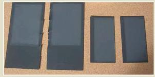
**Above**: After 2000 hours of UV testing the New Zealand product showed no evidence of degradation compared with the imported product (below) tested under the same conditions. Photographs used with the permission of NZMRM.
